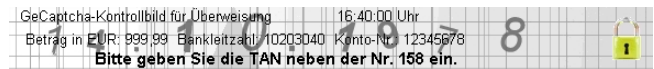
Figure 2: A GeCaptcha image. The big digits in the background compose the user’s birthday. English translation of the three text lines: Line 1 – “GeCaptcha control picture for transfer”; Line 2 – “Amount in EUR: 999,99 Bank code: 10203040 Account Nr.: 12345678”; Line 3 – “Please enter the 158th TAN”.
