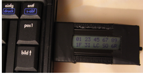
Fig. 4. One prototype USB-token running the hPIN user authentication step.
