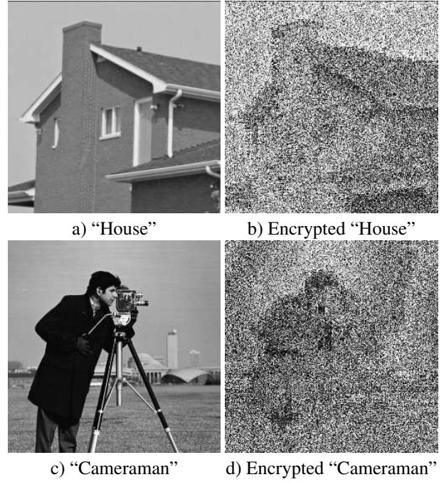
Figure 2: Two natural images, “House” and “Cameraman”, encrypted by TDCEA, with (\alpha, \beta) = (5, 1) , x(0) = 33578/2^{17} \approx 0.2562 and \mu = 129518/2^{15} \approx 3.9526
